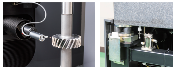
※1 簡易測定 歯車端面粗さ測定、内径粗さ測定 Manual measurement: Surface Measurement, Inner Surface Measurement
