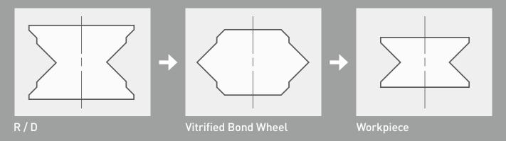
Through truing and dressing a grinding wheel to its correct form, roller dresser sustains the wheels grinding efficiency and accuracy and maintains productivity as well as quality in mass production.
