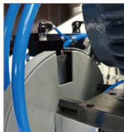
◎ Double V Block Cut 2 bars. Precisely Loading to V Block Movable.
